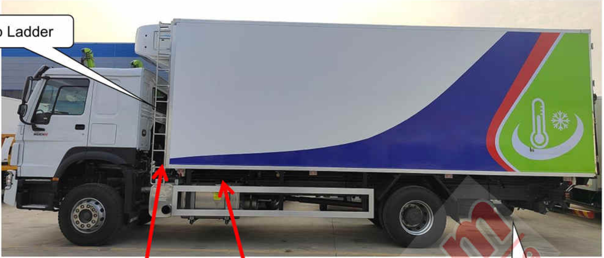
Right View: Refrigerator Body and external power source
